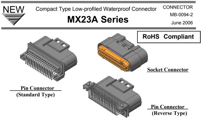
MX23A connector can be used for wide range water proof equipment including automobiles, motorcycles and so on. This connector has high environmental capability with waterproof structure by sealing in its mating area and by grommet in its wire crimping area for full protection against water. Reverse type pin connector (with pins facing up) is also available in consideration of mounting space.
