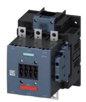
power contactor, AC-3 150 A, 75 kW / 400 V AC (50-60 Hz) / DC operation 110-127 V AC/DC auxiliary contacts 2 NO + 2 NC lateral, permanently mounted 3-pole, frame size S6 busbar connections drive: conventional
