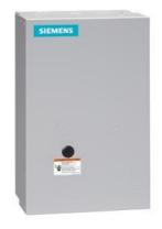
Mechanically held lighting contactor, Contactor amp rating 100A, 0 N.C. / 4 N.O. poles, 110VAC 50HZ/120VAC 60HZ coil, Non-combination type, Enclosure NEMA type 1, Indoor general purpose use
