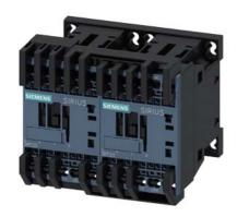
Reversing contactor assembly AC-3,4 kW/400 V,AC48 V,50/60 Hz 3-pole, Size S00 Spring-type terminal electrical and mechanical interlock
