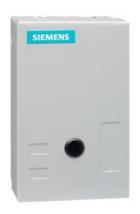
Electrically held lighting contactor, Contactor amp rating 30A, 0 N.C. / 4 N.O. Poles, 198VAC 50HZ/208VAC 60HZ coil, Non-combination type, (no disconnect device), Enclosure NEMA type 1, Indoor general purpose use
