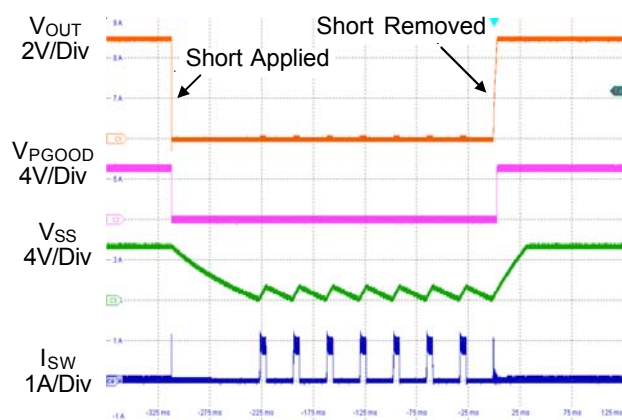
Figure 3. Short Circuit Protection and Recovery
