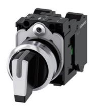
Selector switch, illuminable, 22 mm, round, metal, shiny, white, selector switch, short, 3 switch positions I-O-II, latching, actuating angle 2x45°, 10:30h/12h/13:30h, with holder, 1 NO, 1 NO, spring-type terminal, Z=20-unit packaging
