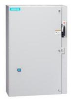
Non-reversing motor starter, Size 3, Three phase full voltage, Solid-state overload relay, OLR amp range 25-100A, 208VAC 60Hz coil, Combination type, 100A fusible disconnect, 100A/250V fuse clip, Enclosure NEMA type 1, Indoor general purpose use, Extra-wide enclosure
