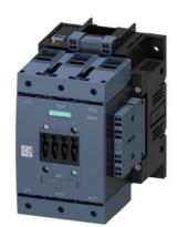
Traction contactor, AC-3 115 A, 55 kW / 400 V Coil 24 V DC x (0.7-1.25) PLC input 24-110 V DC Auxiliary contacts 2 NO + 2 NC 3-pole size S6 with box terminals Coil connection: Spring-type terminal
