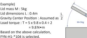
■ When connecting the rotating shaft to other parts, please ensure a tight fit between them. Without a tight fit, the lid will not slow down properly when closing. The corresponding dimensions for fixing the rotating shaft and the main body are as follows.
