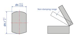
Recommended dimensions for mounting a rotating shaft
