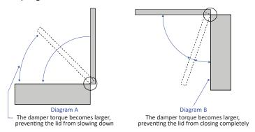
The angle in which the damper torque becomes large can be customized by modifying the inside orifice
