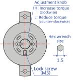
The direction in which torque is generated varies according to the model. Please select the appropriate model for your purpose
