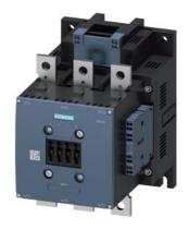
power contactor, AC-3 265 A, 132 kW / 400 V AC (50-60 Hz) / DC operation 440-480 V AC/DC auxiliary contacts 2 NO + 2 NC 3-pole, frame size S10 busbar connections drive: conventional spring-loaded terminal
