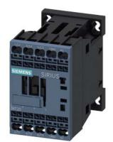
Contactor, AC-3, 7.5 KW / 400 V, 1 NO, 110 V AC, 50 Hz, 120 V, 60 Hz, 3-pole, Size S00 Spring-type terminal
