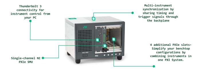
The PXI SMU Bundles features SMUs with 4-quadrant operation, ranges up to  $\pm$  200V and  $\pm$  3A, and sensitivity as low as 100fA. PXI Source Measure Units (SMUs) combine power, precision, and speed into a single instrument. Use the same instrument for both high-power sweeps and low-current measurements and take advantage of a high-speed update rate and sampling rate to use the instrument in non-traditional ways, such as generating and measuring a waveform.
