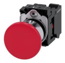
Mushroom pushbutton, 22 mm, round, metal, shiny, red, 40mm, latching, pull-to-unlatch mechanism, with holder, 1 NC, spring-type terminal, with laser labeling, upper case
