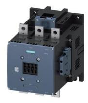
power contactor, AC-3 400 A, 200 kW / 400 V AC (50-60 Hz) / DC operation 21-27 AC/DC, 3 V auxiliary contacts 2 NO + 2 NC 3-pole, frame size S12 busbar connections drive: electronic with PLC interface 24 V DC screw terminal
