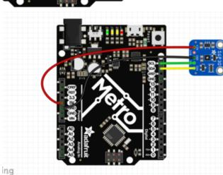
Board 5V to Sensor Vin (red wire on STEMMA QT version). (Metro is a 5V logic chip)
