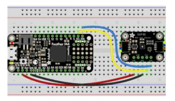
Board 3.3V to sensor Vin (red wire on STEMMA QT version) (Feather is 3.3V logic)
