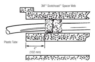
3.5 Wrap the foam strip around the cable and insert it into the duct. The foam strip should be flush with the duct entrance and should fit snugly between the cable and duct.
