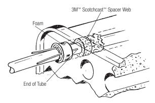
3.7 Mix one bag of sealant foam according to the instructions on the bag.
