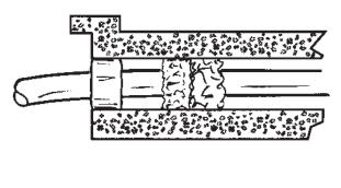
3.6 Cut one of the 12" (305 mm) plastic tubes in half making two 6" (152 mm) tubes. Insert the 6" tubes within the last wrap of the foam strip. Position one tube at the 12 o'clock position and the other at either the 3 or 9 o'clock position.
