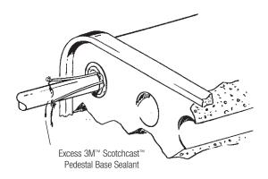
*Note: Once the compound has been injected, the cable should not be moved for at least one hour.*
