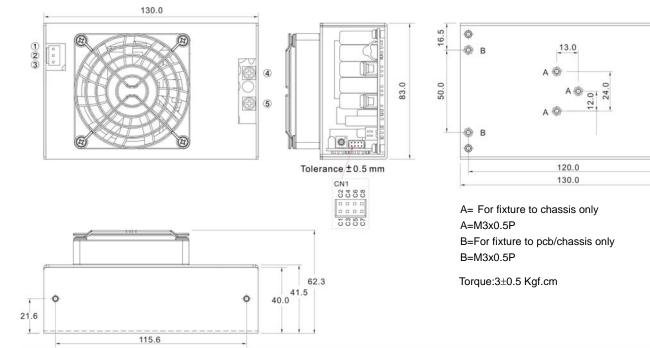
\*U Case T=1.5mm Customer is advised to screw into the threads no more than 1.5mm
