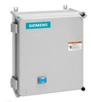
Non-reversing motor starter, Size 2 1/2, Three phase full voltage, Amb. compensate bimetal OLR, Contactor amp rating 60A, Non-combination type, Enclosure type 4X fiberglass, Water/dust tight noncorrosive
