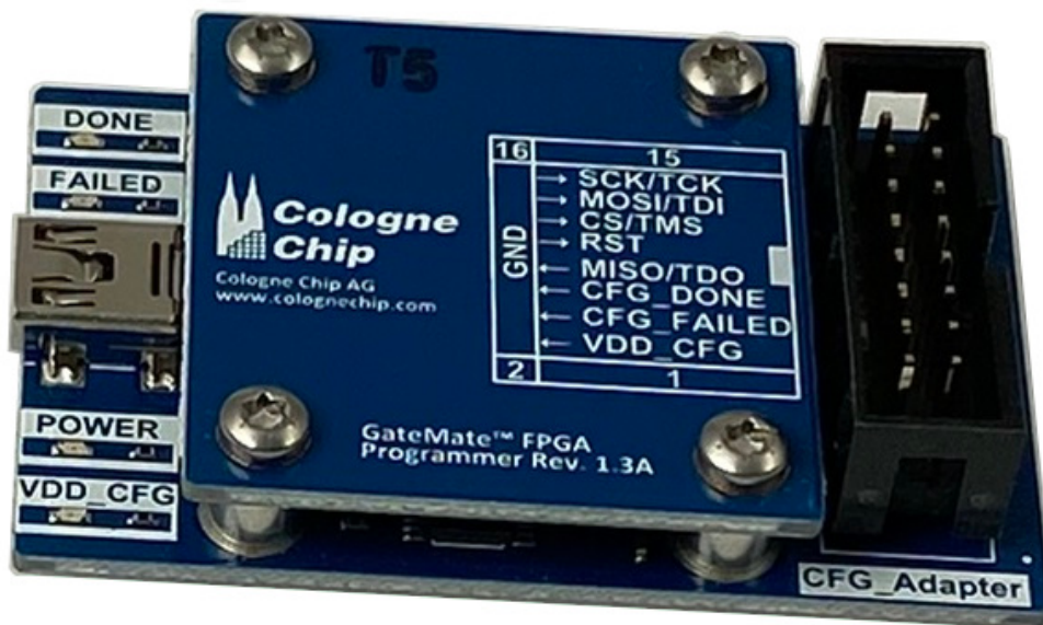
Figure 1.1: Top view of the GateMate™ FPGA Programmer (including module cover)
