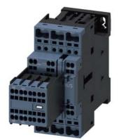
power contactor, AC-3 9 A, 4 kW / 400 V 2 NO + 2 NC, 230 V AC, 50 Hz 3-pole, Size S0 Spring-type terminal Removable auxiliary switch
