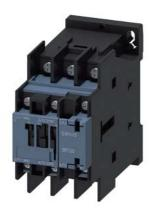
power contactor, AC-3 25 A, 11 kW / 400 V 1 NO + 1 NC, 100 V AC, 50 Hz, 100-110 V, 60 Hz, 3-pole, Size S0, ring cable lug connection
