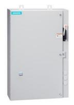
Non-reversing motor starter, Size 1, Three phase full voltage, Solid-state overload relay, OLR amp range 10-40A, 110V 50Hz / 120V 60Hz coil, Combination type, 60A fusible disconnect, 60A/250V fuse clip, Enclosure NEMA type 4/12, Water/dust tight for outdoors, Extra-wide enclosure
