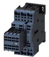
power contactor, AC-3 25 A, 11 kW / 400 V 2 NO + 2 NC, 110 V AC, 50 Hz, 3-pole, Size S0 Spring-type terminal Removable auxiliary switch
