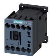
Power contactor, AC-3 9 A, 4 kW / 400 V 1 NO, 12 V DC 3-pole, Size S00 screw terminal
