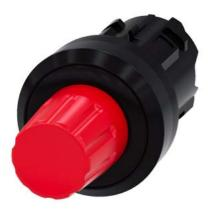
Stop button, 22 mm, round, plastic, red, pushbutton raised, latchable after pushing in by rotating clockwise, unlatch by rotating counter-clockwise
