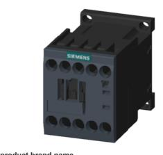
Power contactor, AC-3 7 A, 3 kW / 400 V 1 NC, 100 V AC, 50 Hz 100-110 V, 60 Hz, 3-pole, Size S00, screw terminal
