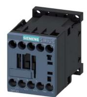
Power contactor, AC-3 9 A, 4 kW / 400 V 1 NO, 400 V AC, 50 Hz 400-440 V, 60 Hz, 3-pole, Size S00, screw terminal
