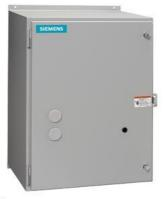
Mechanically held lighting contactor, Contactor amp rating 200A, 0 N.C. / 3 N.O. poles, 110VAC 50HZ/120VAC 60HZ coil, Non-combination type, Enclosure NEMA type 12, Dust/drip proof for indoors
