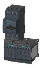
Load feeder fuseless, Reversing duty 400 V AC, Size S00 0.28...0.40 A 230 V AC screw terminal for installation on standard mounting rail (also fulfills type of coordination 1) Type of coordination 2, Iq = 150 kA 1 NC (contactor)
