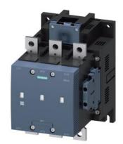
vacuum contactor, AC-3 225 A, 110 kW / 400 V AC (50-60 Hz) / DC operation 96-127 V AC/DC auxiliary contacts 2 NO + 2 NC 3-pole, frame size S10 busbar connections drive: electronic with PLC interface 24 V DC
