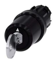
key-operated switch Siemens, 22 mm, round, plastic, lock number SSG10, with 2 keys, 3 switch positions I-O-II, latching, actuating angle  $2x45^{\circ}$ , 10:30h/12h/13:30h, key removal I+O+II
