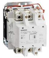
Mechanically held lighting contactor, Contactor amp rating 200A, 0 N.C. / 5 N.O. poles, 220VAC 50HZ/240VAC 60HZ coil, Non-combination type, Enclosure NEMA type (open), No enclosure
