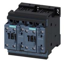
Reversing contactor assembly for 3RA27 AC-3, 11 kW/400 V, 24 V DC 3-pole, Size S0 screw terminal electrical and mechanical interlock 2 NO integrated, with voltage tap
