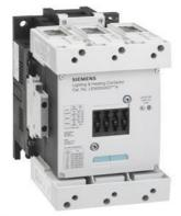
Electrically held lighting contactor, Contactor amp rating 300A, 0 N.C. / 3 N.O. Poles, 277VAC 60HZ coil, Non-combination type, (no disconnect device), Enclosure NEMA type (open), No enclosure
