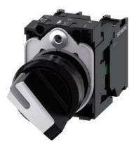
Selector switch, illuminable, 22 mm, round, plastic, white, selector switch, short, 2 switch positions O-I, latching, 10:30h/13:30h, with holder, 1 NO, 1 NC, screw terminal, with laser labeling, upper case and lower case, always upper case at the beginning of the word
