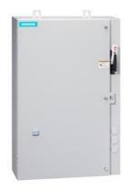
Non-reversing motor starter, Size 2 1/2, Three phase full voltage, Solid-state overload relay, OLR amp range 25-100A, Combination type, 100A non-fusible disconnect, Encl NEMA type 4X 304 S-Steel, Water/dust tight noncorrosive, Standard width enclosure
