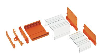
Extruded profile for locking base system, length: 2000 mm, lower part, width: 84 mm, PCB width: 68 or 73 mm,, colour: orange, Note: required profile length = PCB length - 4.5 mm
