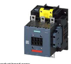
Power contactor, AC-3 185 A, 90 kW / 400 V Coil AC 50/60 Hz and DC 96-127 V x (0.8-1.1) F-SPS input 24 V DC 3-pole size S6 Auxiliary contacts 2 NO + 2 NC permanently mounted Main circuit: Busbar Control and auxiliary circuit: Screw terminal
