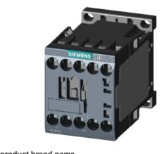
Power contactor, AC-3 9 A, 4 kW / 400 V 2 NO + 2 NC 220 V AC, 50 Hz/240 V, 60 Hz 4-pole Size S00 screw terminals
