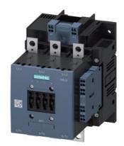
power contactor, AC-3 115 A, 55 kW / 400 V AC (50-60 Hz) / DC operation 240-277 V AC/DC auxiliary contacts 2 NO + 2 NC 3-pole, frame size S6 busbar connections drive: conventional spring-loaded terminal
