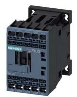
Power contactor, AC-3 9 A, 4 kW / 400 V 1 NO, 48 V DC, 3-pole, Size S00 Spring-type terminal
