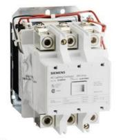
Mechanically held lighting contactor, Contactor amp rating 200A, 0 N.C. / 4 N.O. poles, 208VAC 60HZ coil, Non-combination type, Enclosure NEMA type (open), No enclosure
