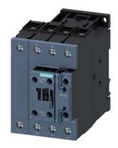
Contactor, 2NO + 2NC, AC-3, 18.5 kW, 110 V AC, 50 Hz, 4-pole, 2NO + 2NC, Size S2, Screw terminal 1 NO + 1 NC integrated
