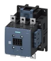
power contactor, AC-3 225 A, 110 kW / 400 V AC (50-60 Hz) / DC operation 380-420 V AC/DC auxiliary contacts 2 NO + 2 NC 3-pole, frame size S10 busbar connections drive: conventional spring-loaded terminal
