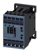
Power contactor, AC-3 16 A, 7.5 kW / 400 V 1 NO, 24 V DC communication-capable, 3-pole Size S00, Spring-type terminals
