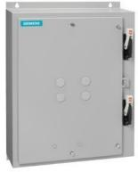
Duplex starter w/ alternator, Size 4, Three phase full voltage, Amb compensate bimetal OLrelay Contactor amp rating 135Amp 110V 50HZ / 120V 60HZ coil, Combination type, Two 200A disconnect switches, Enclosure NEMA type 1, Indoor general purpose use
