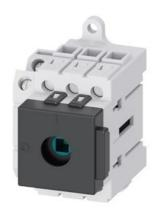
Load disconnector 3LD3, lu 16 A Main switch 3-pole Rated operating capacity at AC-23 A at 400V 7.5kW Installation in distribution boards, Basic switch without Knob-operated mechanism with auxiliary switch 1OE + 1S
