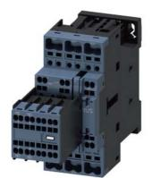
power contactor, AC-3 25 A, 11 kW / 400 V 2 NO + 2 NC, 220 V AC, 50 / 60 Hz, 3-pole, Size S0, Spring-type terminal Removable auxiliary switch
