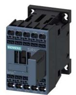
power contactor, AC-3 12 A, 5.5 kW / 400 V 1 NC, 24 V DC 0.85-1.85\* US, with varistor plugged on, 3-pole size S00, spring-type terminal not expandable with auxiliary switch
